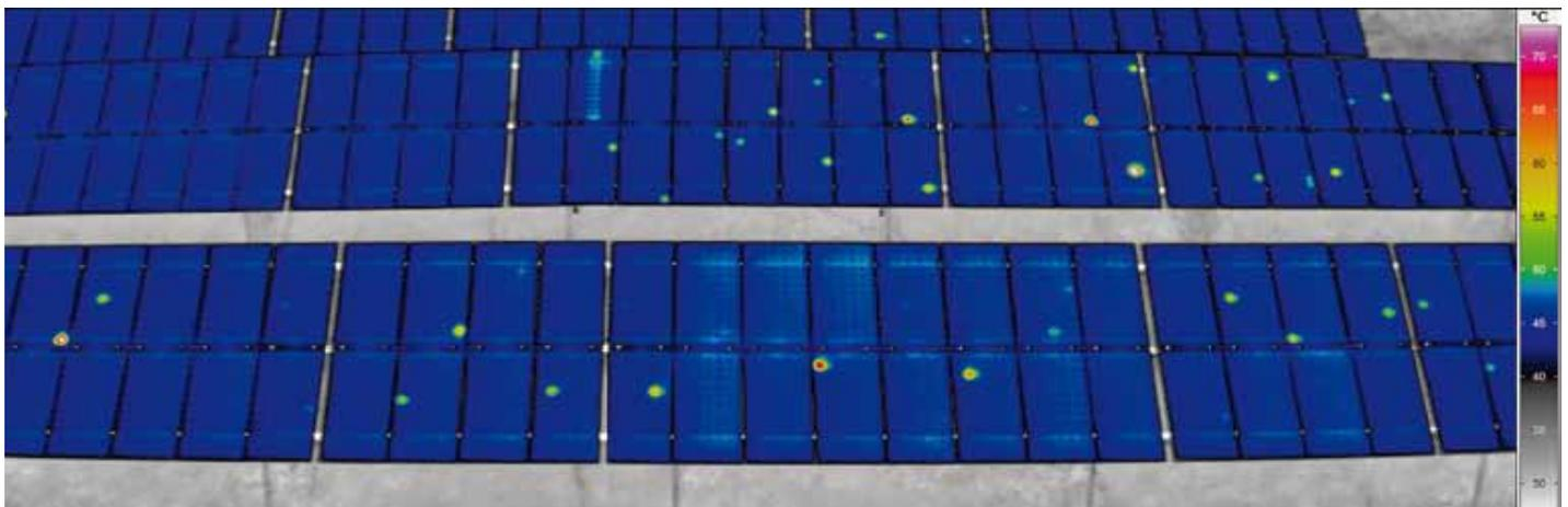
Thermal picture of a PV generator in a MW plant. Fortunately, not every generator displays so many warm cells. But not every warm cell means a defect. Long-time experience is necessary to distinguish the problematic abnormalities from the ones that do not matter.
