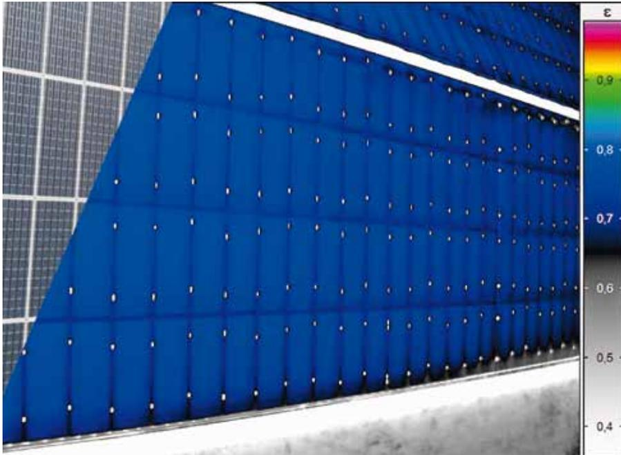
Superimposed visual image on the left and infrared image on the right: Missing or incorrectly positioned module clamps are the most frequent but not by any means the only faults that thermography can reveal in the mounting system. Deeper anomalies can also be detected and explained.
