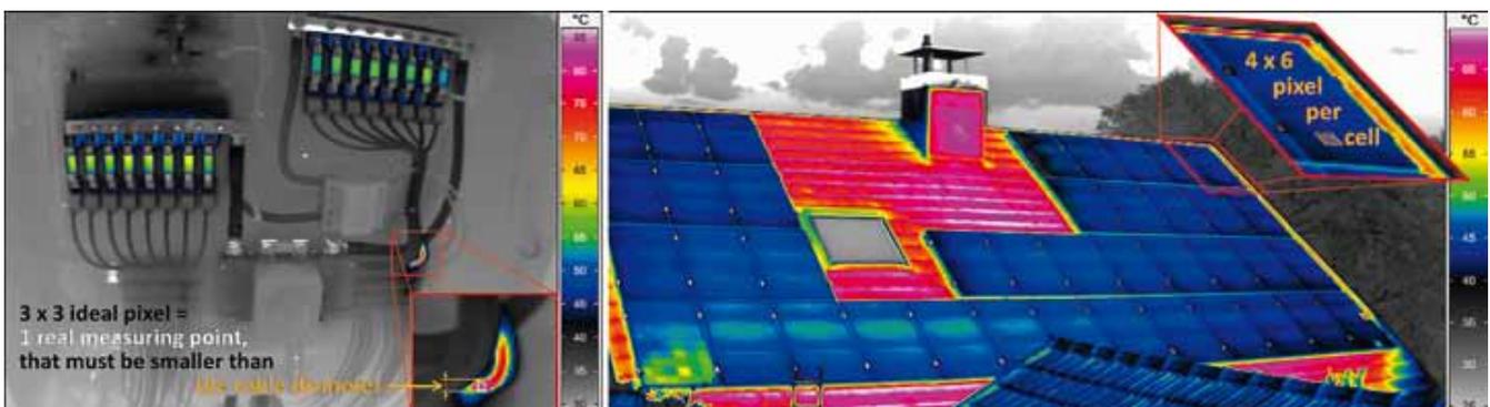
Recommendation for geometric resolution in electrical and PV thermography.
